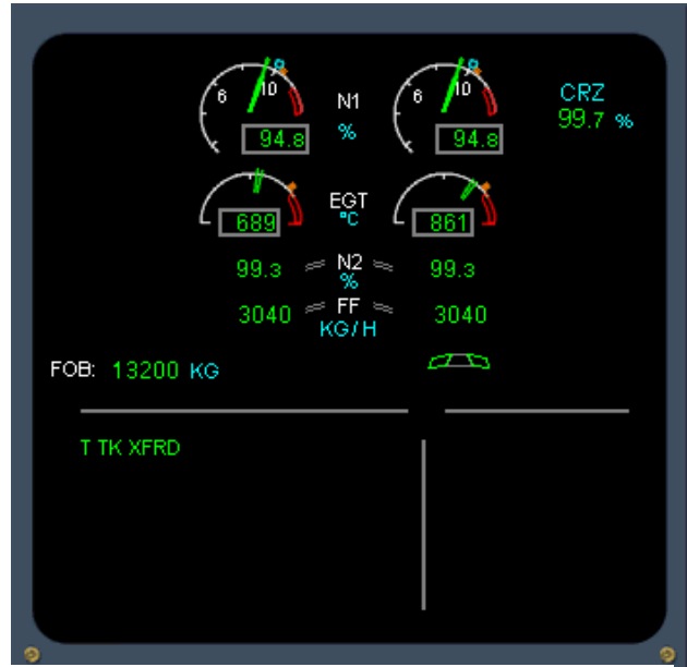
Figure 5 - E/WD & Trim Tank Transferred Memo
