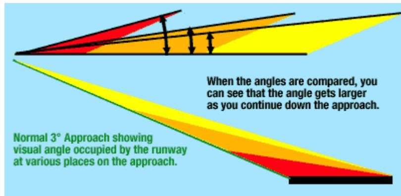
**Figure 4: The visual angle subtended by the runway during a normal three-degree approach should get larger and larger as you continue the approach.**
