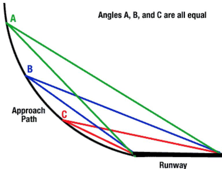
Figure 6: If the pilot keeps the visual angle subtended by the runway constant, the approach path will be an arc.
