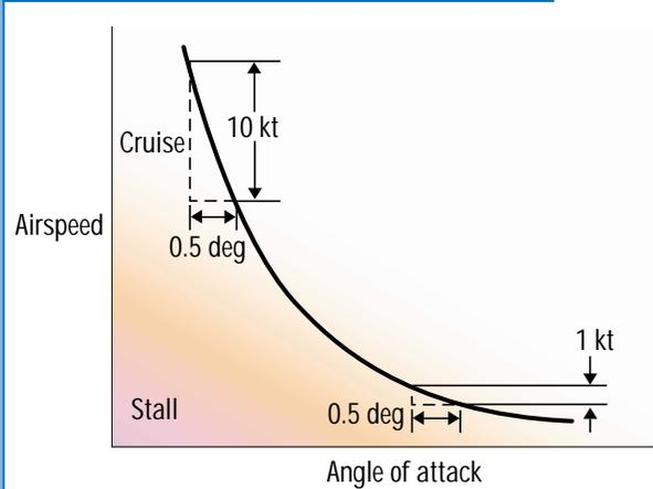
An error in AOA corresponds to a much higher error in airspeed or gross weight at high speeds than at low speeds. For a mid-sized airplane, such as the 757-200, a 0.5-deg error in AOA results in the following errors:
