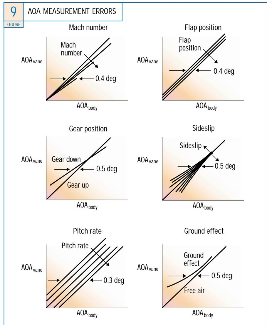
For the most part, the effects discussed above can be compensated for and, depending on the airplane, many have been. It should be noted, however, that each correction has its own inherent uncertainty and can also cause erroneous readings if the input data is incorrect.
