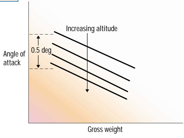
can be seen that the optimal long-range cruise Mach number does not vary significantly as gross weight (hence, lift and AOA) changes. Superimposed on this chart are two lines of constant AOA. It is apparent that flying a constant AOA will not yield optimal performance. If a flight crew tried to fly a target AOA and there was an error of as little as 0.5 deg, the penalty in fuel mileage could be 3 percent or more.
