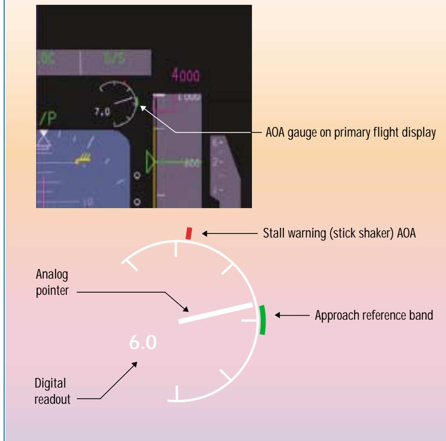
to cruise. The position of the amber and red bands is always a function of AOA margin to stall warning.
