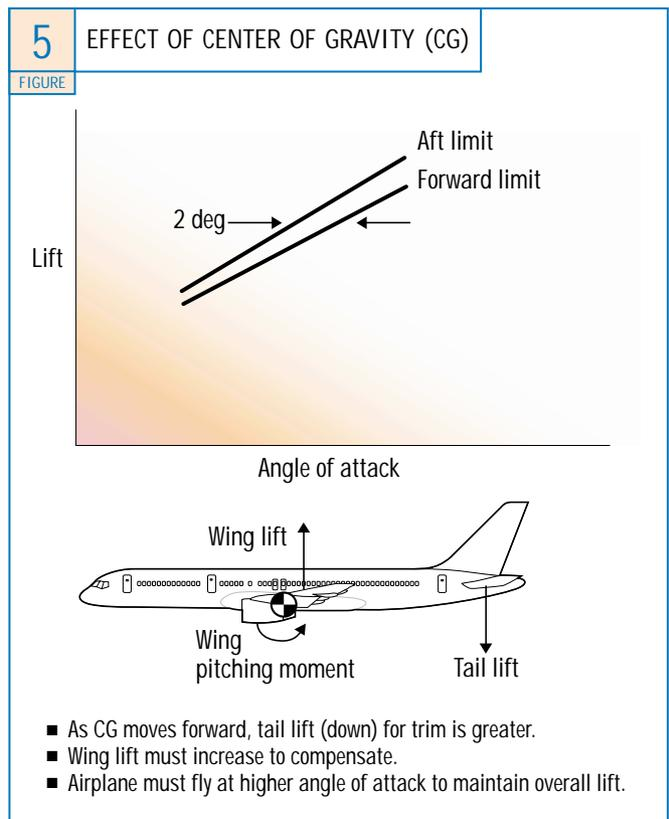
that the wing must provide enough lift to compensate for the download on the tail in addition to the weight of the airplane. Note that the AOA of stall is not changed, but the lift required of the wing is greater, and therefore the stall speed is increased.
