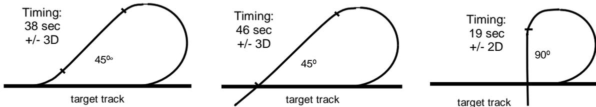
The "target track" in these figures is for example the runway track. Turns are standard rate-one turns at 25° angle of bank. The depicted courses are in fact tracks, therefore corrected for possible drift.
