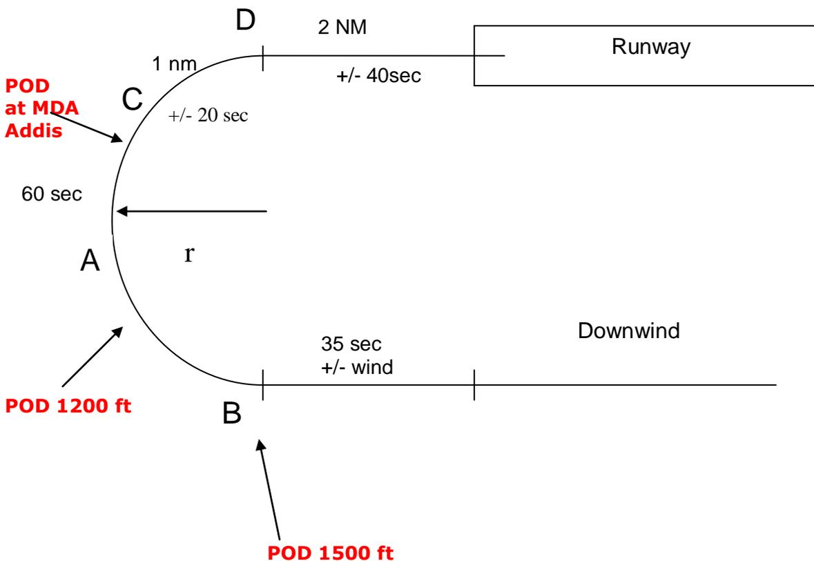
Some pilots tend to use the NAV display to verify the correct downwind distance while circling. However the large difference in TAS between airports on sea level and high altitude airports like Addis will cause a significant difference in downwind distance. From the timing used during circling the exact distance from the runway on downwind can be calculated as follows:
