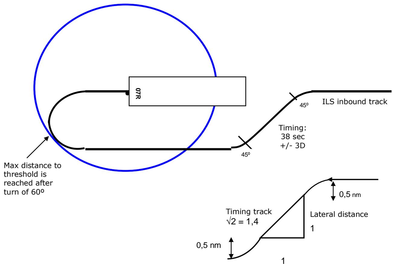
Timing : The airplane performs two turns with a 45° track change. Both turns will create a lateral displacement of 1 nm in total. The displacement on the timing track can be calculated as follows: If TAS is 180 kts this corresponds to 3 NM/Min. Timing 38 secs = 1,73 NM
