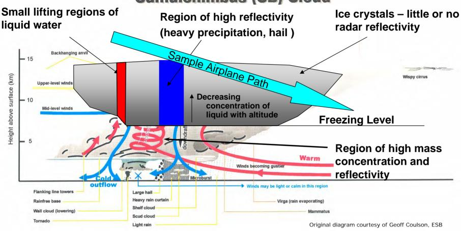
Above the freezing level, the convective cloud may be dominated by small ice particles, invisible to onboard weather radar
