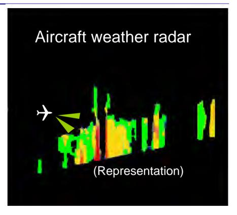
Flight in ice crystals will look like visible moisture, but will not produce significant radar returns. Isolated high reflectivity targets ahead may be detected.
