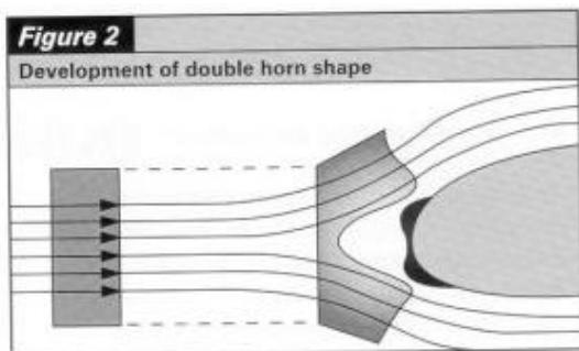
This starts the double horn shape, which is a divergent process and which is further enhanced by ram effect (figure 2). But if the droplets are very heavy, as in the case of freezing rain, deflection is limited, and ice accretion takes place in an arc shape (figure 3).
