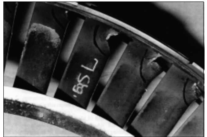
Left-engine seventh-stage-compressor stator damage. (Photo: Finnish Accident Investigation Board)
