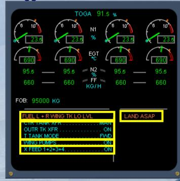
✓ FUEL L+R WING TK LO LVL is inhibited below 800 feet AGL
