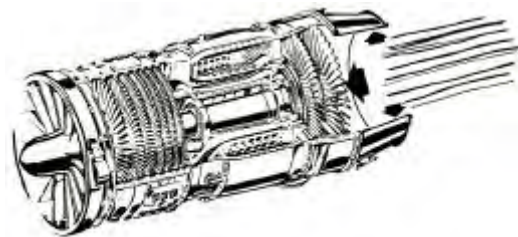
Fig 4 showing turbine engine as a cylinder of turbomachinery with unbalanced forces pushing forward.
