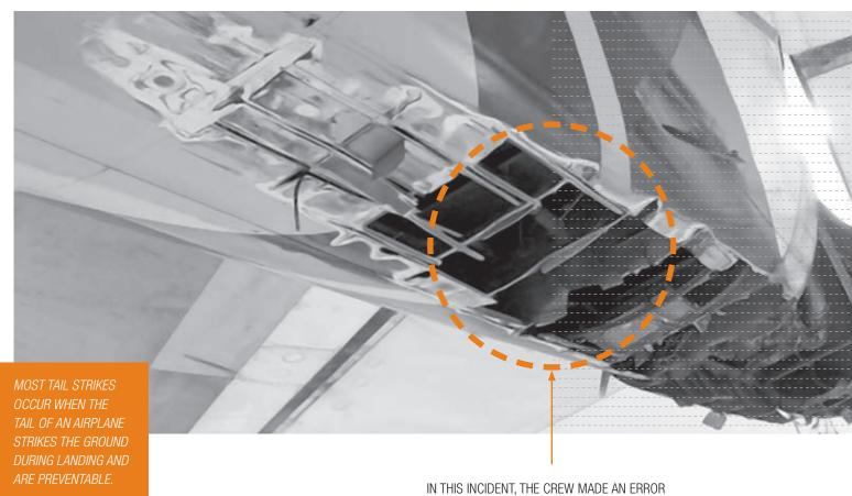
AND CALCULATED TAKEOFF DATA INCORRECTLY. THIS RESULTED IN AN EARLY ROTATION.
