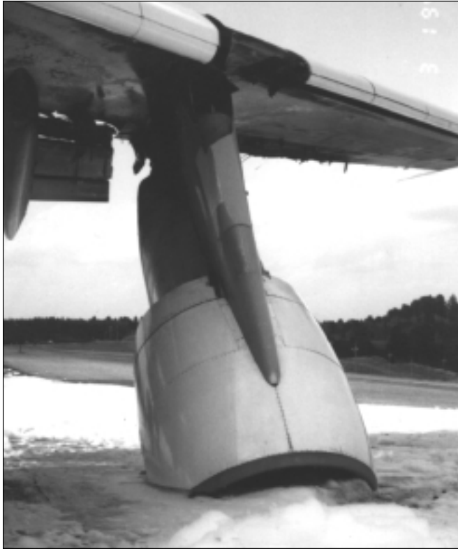
Northwest Airlines Boeing 747's No. 1 engine and pylon rotated downward during the landing roll-out. The lower forward part of the engine cowling was ground away by dragging on the runway.
